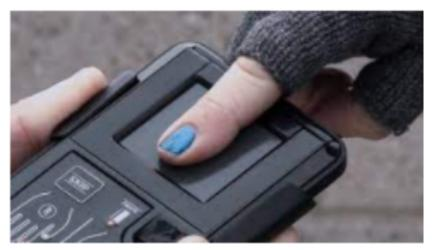
Figure 12.2 Biometric Fingerprint Scanner
