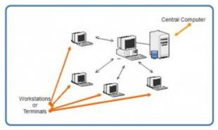
Figure 6.1. Example of a centralized database system.
