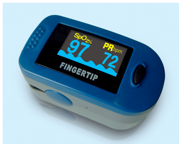
Figure 9.9.1: A fingertip pulse oximeter
