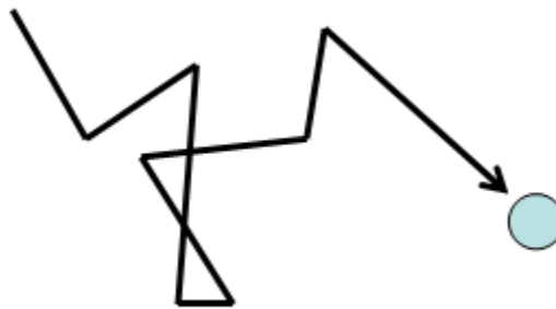
Figure 6.13 “Particle Mean Free Path.” Stylized depiction of the path travelled by a gas particle during diffusion. Other particles have been omitted for clarity.
