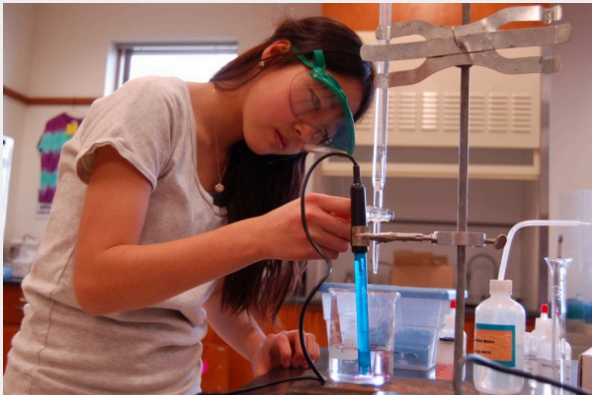
When a student performs a titration, a measured amount of one solution is added to another reactant. "Chemistry titration lab" by Kentucky Country Day is licensed under the Creative Commons Attribution-NonCommercial 2.0 Generic.
