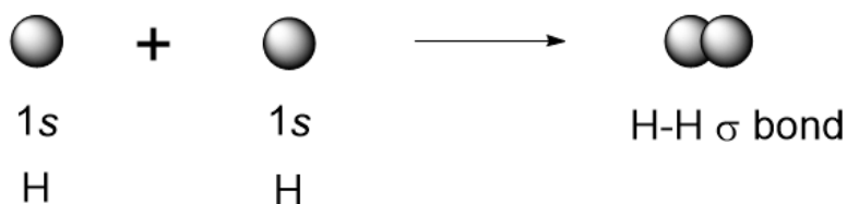
Figure 9.6. A diagram showing the overlap of s orbitals of two hydrogen atoms to form H_2 .
