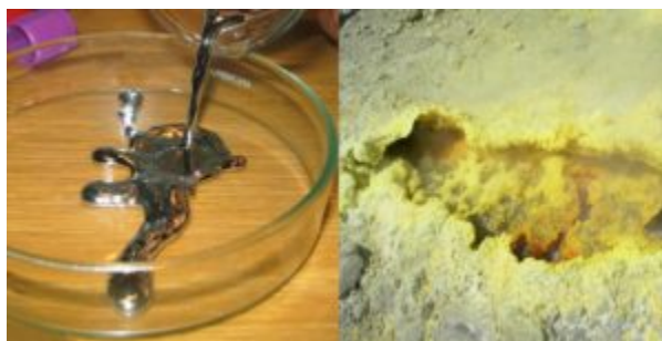
Figure 1.5 “Semimetals.” On the left is some elemental mercury, the only metal that exists as a liquid at room temperature. It has all the other expected properties of a metal. On the right, elemental sulfur is a yellow nonmetal that usually is found as a powder.
