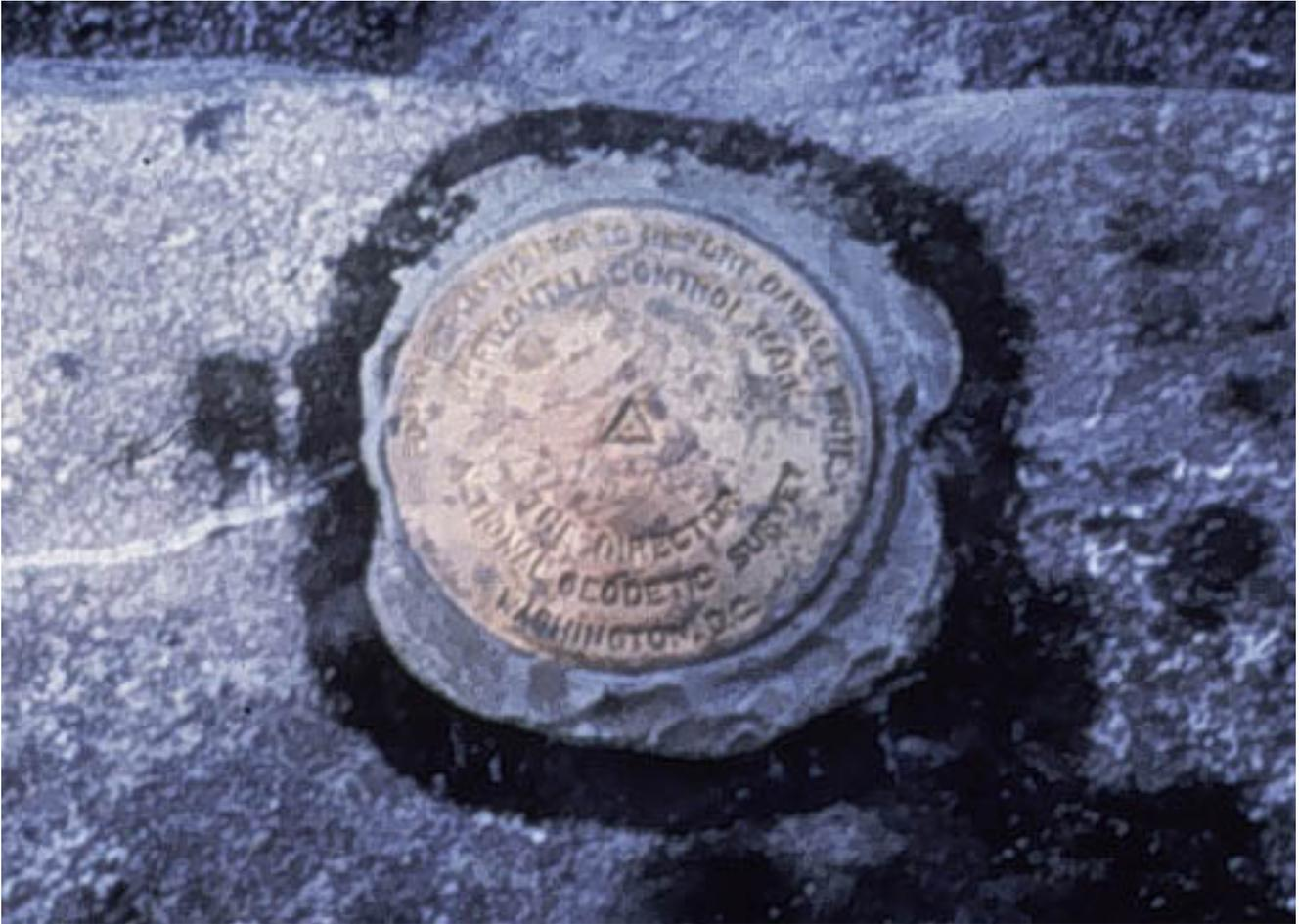
In the U.S., high-order horizontal control point locations are marked with permanent metal “monuments” like the one shown above. The physical manifestation of datum is a network of control point measurements (National Geodetic Survey, 2004).
