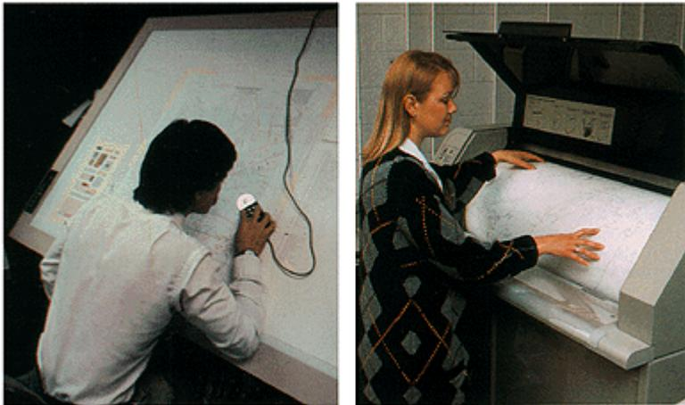
Vector digitizing with a tablet (left); raster digitizing with a drum scanner (right) (USGS).
