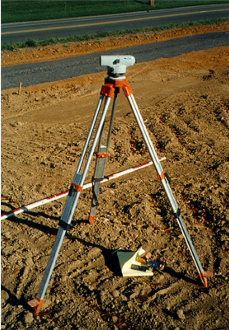
A level used for determining elevations.
