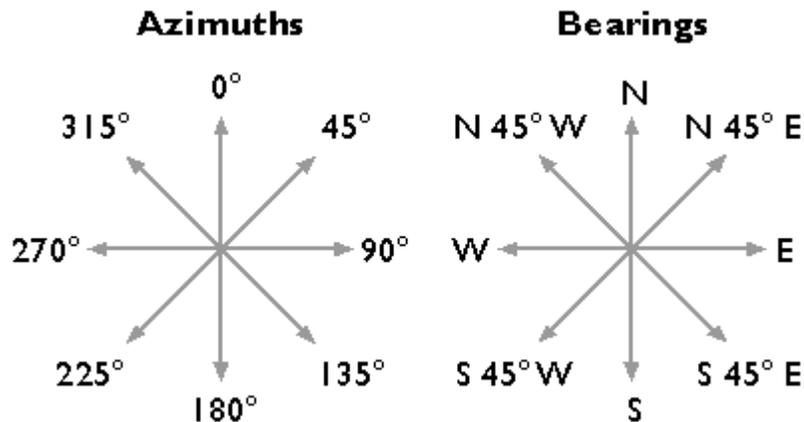
Azimuths and bearings.
