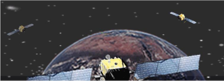
Positioning signals broadcast from three Global Positioning System satellites are received at a location on Earth. (U.S. Federal Aviation Administration, 2007b)
