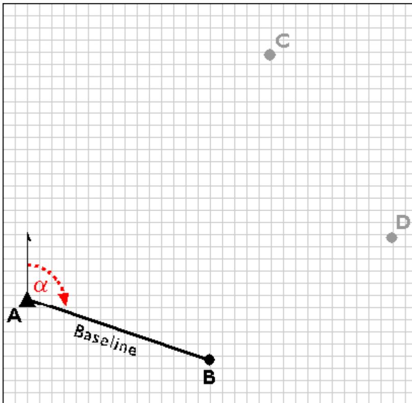
Establishing a second control point (B) in a trilateration network.
