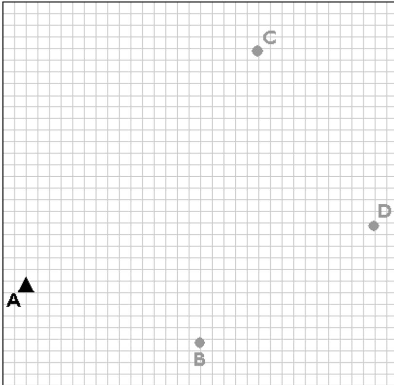
The purpose of a control survey is to establish new horizontal control points (B, C, and D) based upon an existing control point (A).
