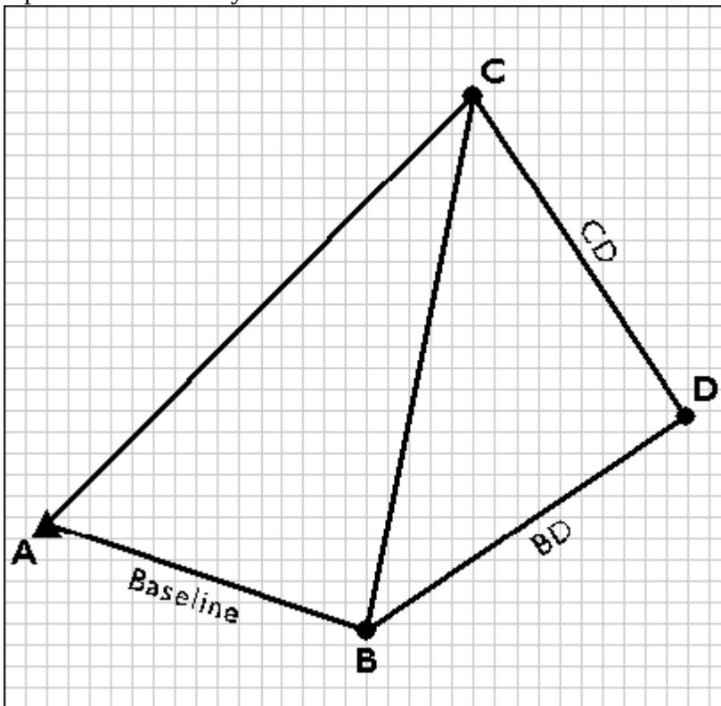
Fixing control point D by trilateration.
