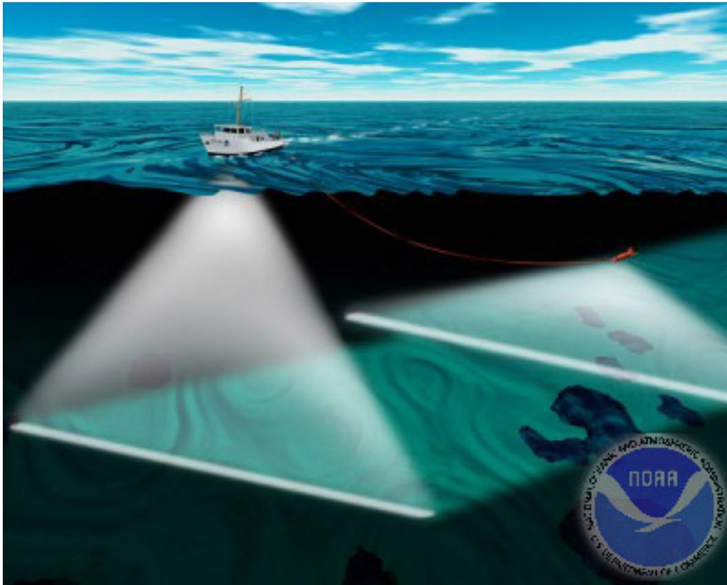
Multibeam and side scan sonar in use for bathymetric mapping. (NOAA, 2002).
