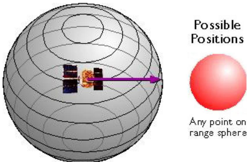
Set of possible positions of a GPS receiver relative to a single GPS satellite. (Adapted from Hurn, 1993).
