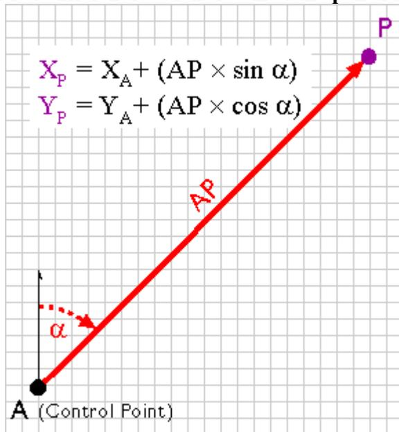
An open traverse. (Adapted from Robinson, et al., 1995)
