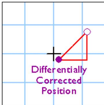
Error correction calculated at the base station is applied to the position calculated by the mobile receiver.
