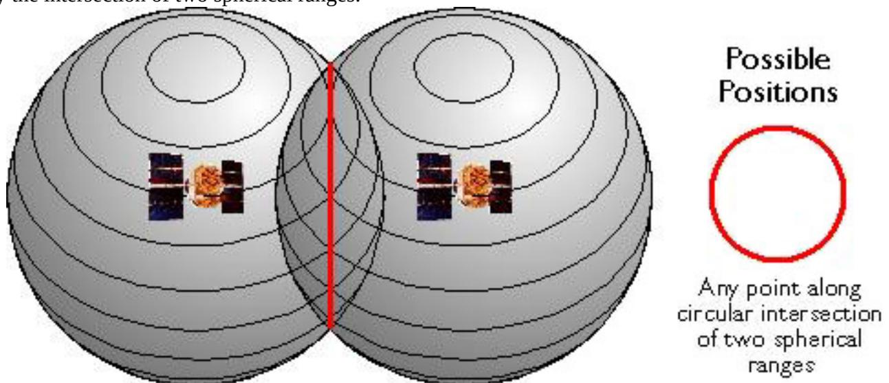
Set of possible positions of a GPS receiver relative to two GPS satellites. (Adapted from Hurn, 1993).
