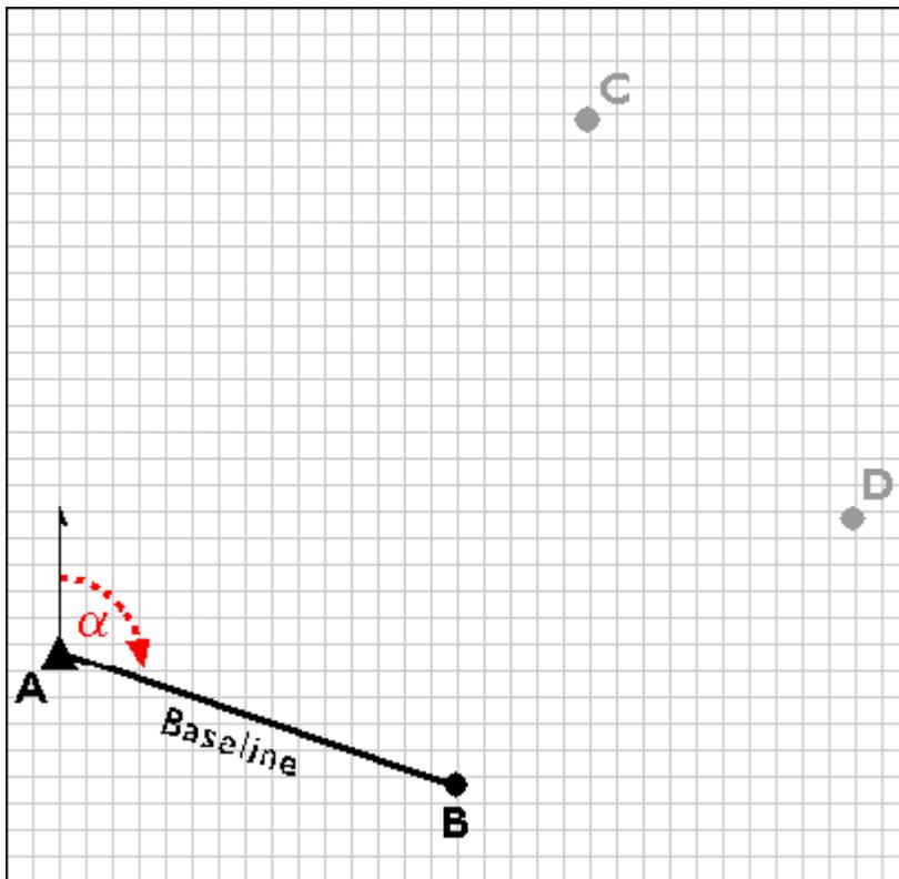
Establishing a second control point (B) in a triangulation network.
