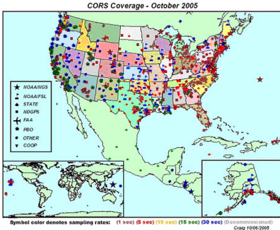
The Continuously Operating Reference Station network (CORS) (Snay, 2005)
