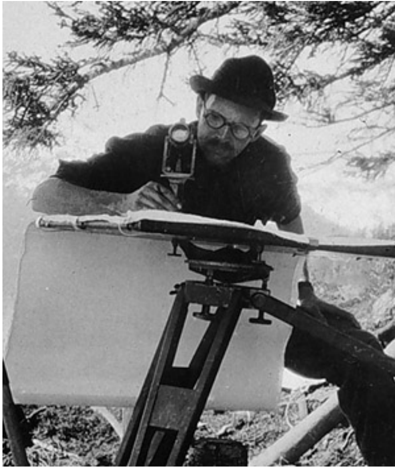
Topographer compiling topographic map using a plane table and alidade (NOAA, 2007).
