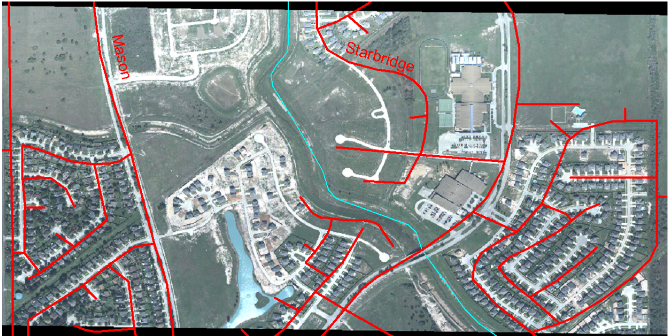
Discrepancy between pre-modernization TIGER/Line file streets (red) and actual geometry of street network shown in an orthorectified aerial image (U.S. Census Bureau n.d).
