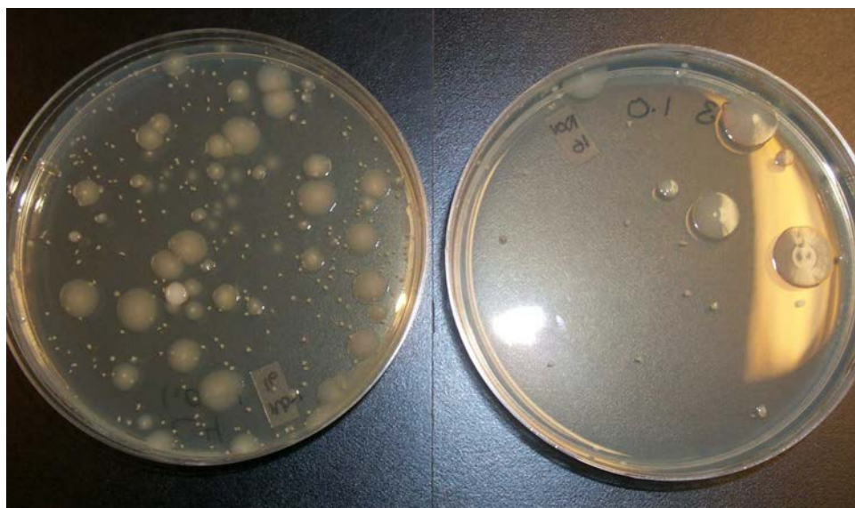
Figure 4 — Counts from the nutrient agar serial dilutions (10 × dilution left; 100 × dilution, right)
