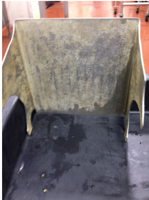
Figure 6 — Biofilm build-up on meat plant equipment before cleaning
