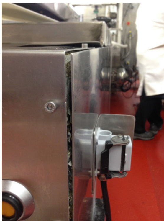
Figure 16 — Soil and food debris found behind the panel cover of this equipment
