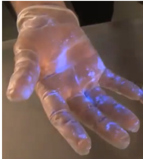
Figure 19 — Glo-germ illuminated by ultraviolet (UV) light on a glove representing areas of contamination on the glove.
