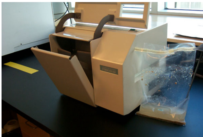
Figure 1 — Food sample after mixing in a stomacher
