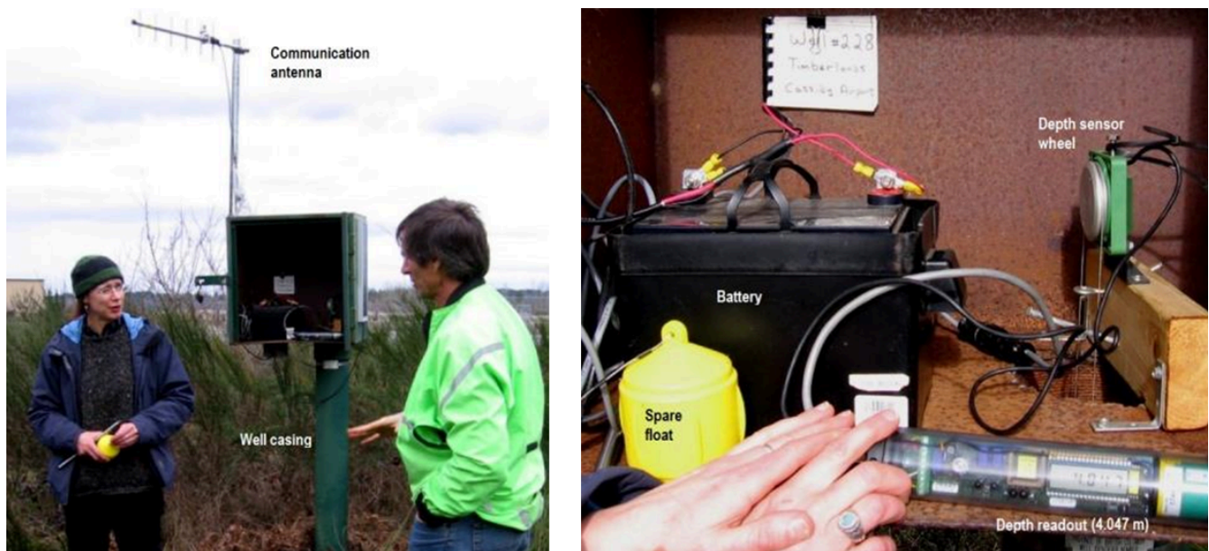
Figure 14.3.5 B.C. observation well 228 near Cassidy, Vancouver Island. The installation also has a solar panel, which is not visible in this view. [Image Description]
