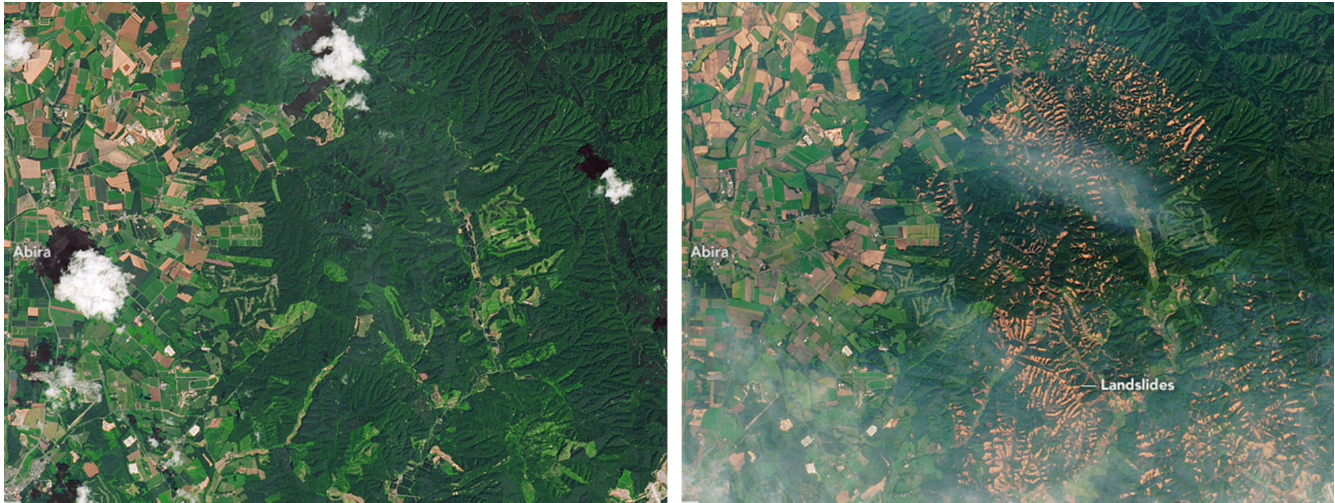
Figure 15.1.7 Slope failures in the Sapporo area of Japan following a typhoon (Sept. 4th, 2018) and earthquake (Sept. 6th, 2018) (Before and after Landsat 8 images: left: July 2017, right: September 2018).
