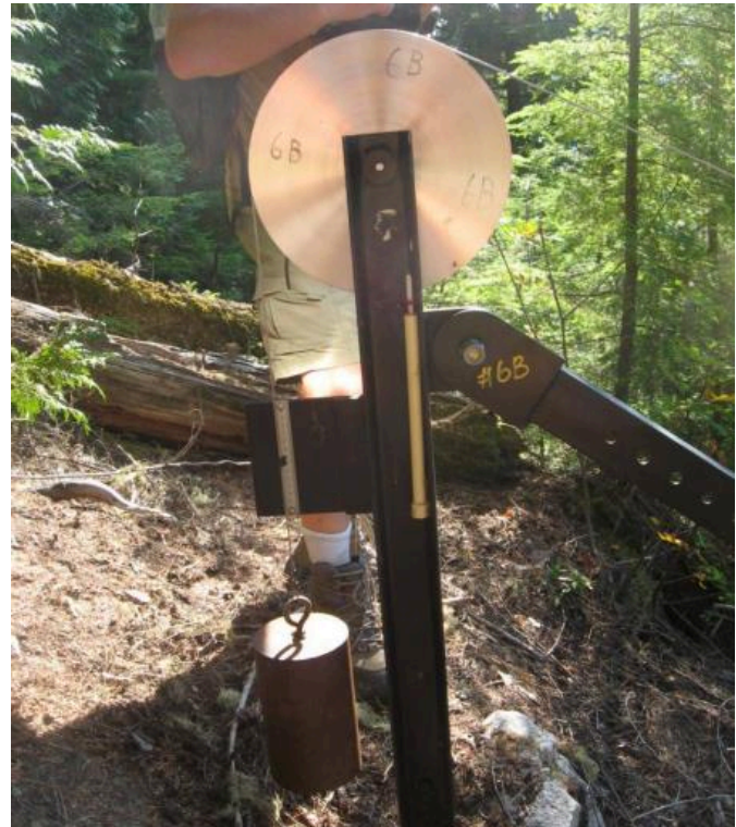
Figure 15.3.3 Part of a motion-monitoring device at the Checkerboard Slide near Revelstoke, B.C. The lower end of the cable is attached to a block of rock that is unstable. Any incremental motion of that block will move the cable, which will be detectable on this device.
