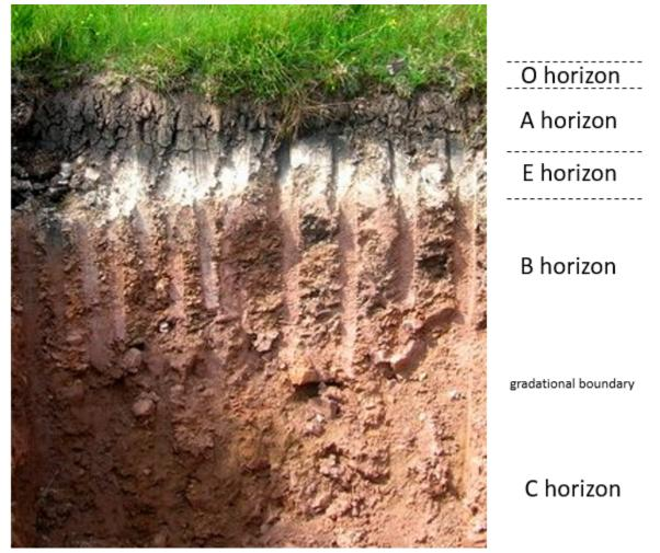
Figure 5.4.3 Soil horizons in a podsol from a site in northeastern Scotland.
