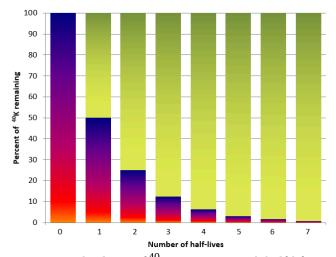
*Figure 8.4.1 The decay of* <sup>40</sup>*K over time. Each half-life is* 1.3 *billion years, so after 3.9 billion years (three half-lives)* 12.5% of the original <sup>40</sup>*K will remain. The red-blue bars represent* <sup>40</sup>*K and the green-yellow bars represent* <sup>40</sup>*Ar.* [*Image Description*]
