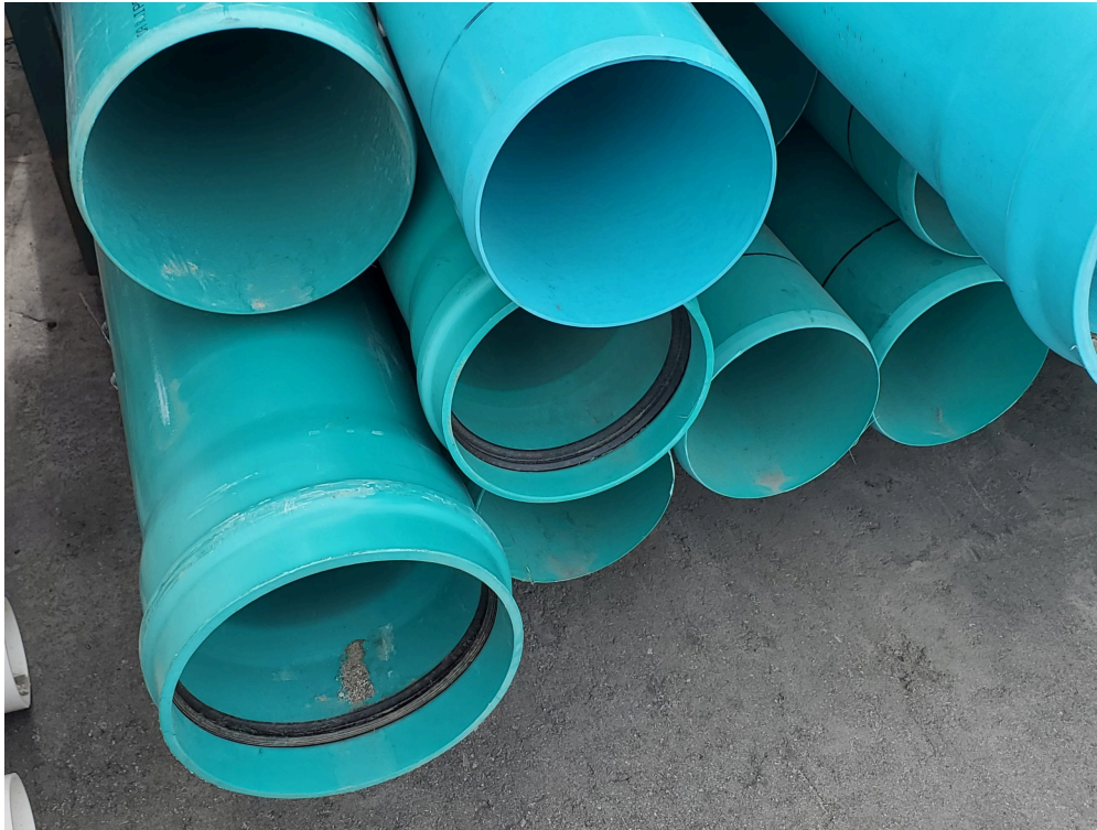
Figure 5 PVC sewer pipe
