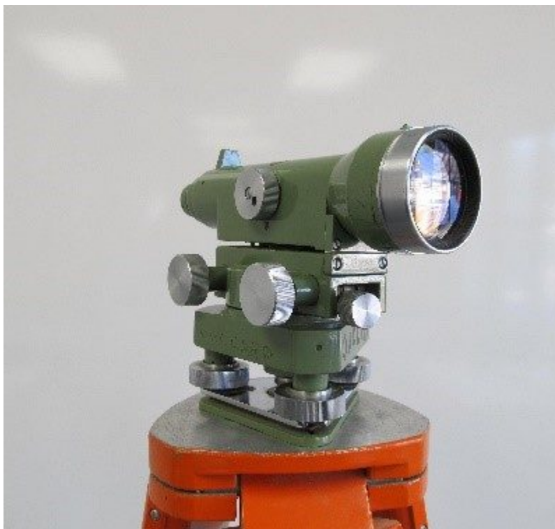
Figure 1 Builders level on tripod
