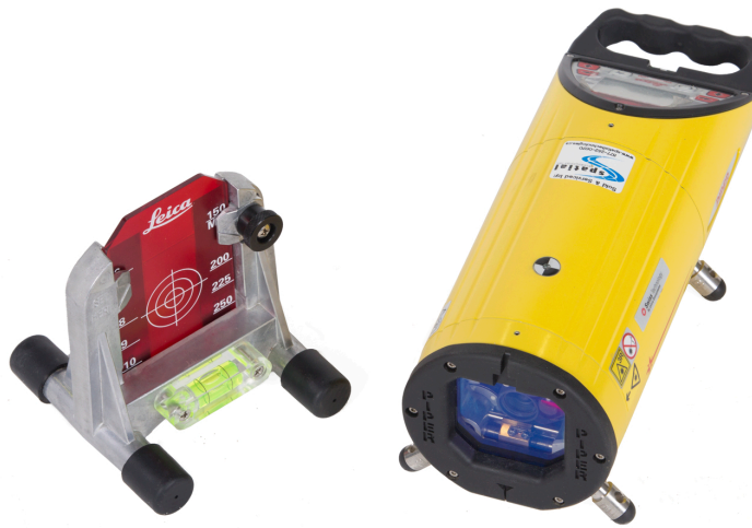
Figure 3 Pipe laser and target for pipe interior
