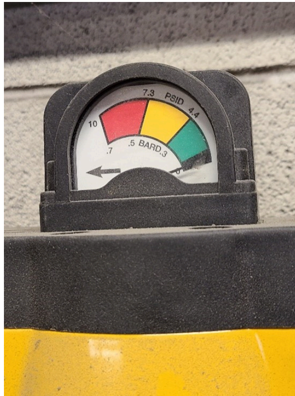
Figure 9 Filter differential pressure indicating gauge
