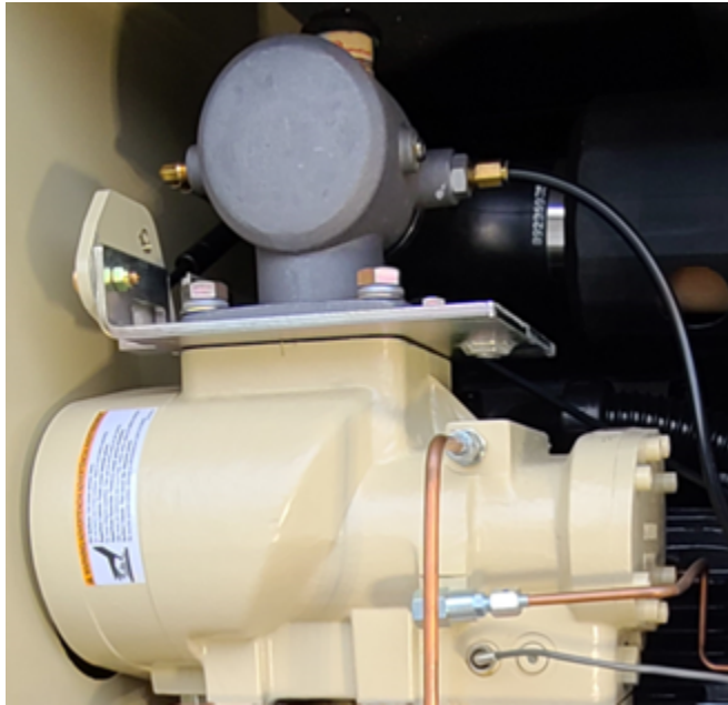
Figure 5 Screw Compressor with inlet/unload valve
