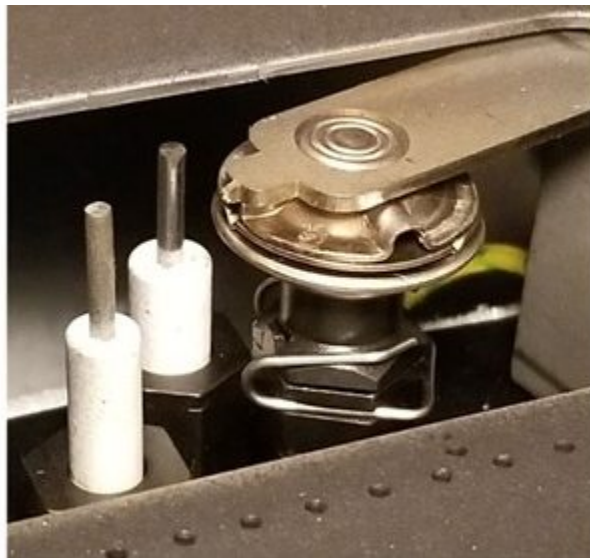
Figure 6 Pilot burner with separate flame rod and spark igniter
