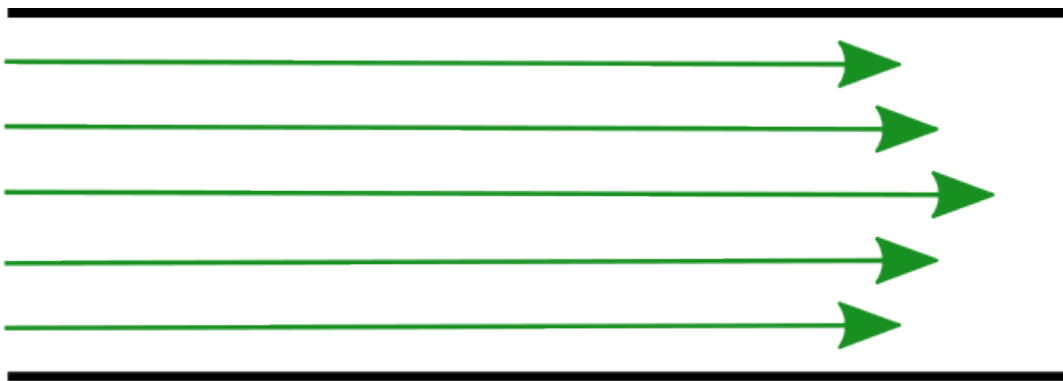
Figure 1 Laminar flow patterns
