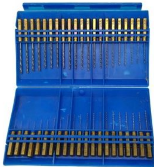
Figure 10 Finger orifice drill set
