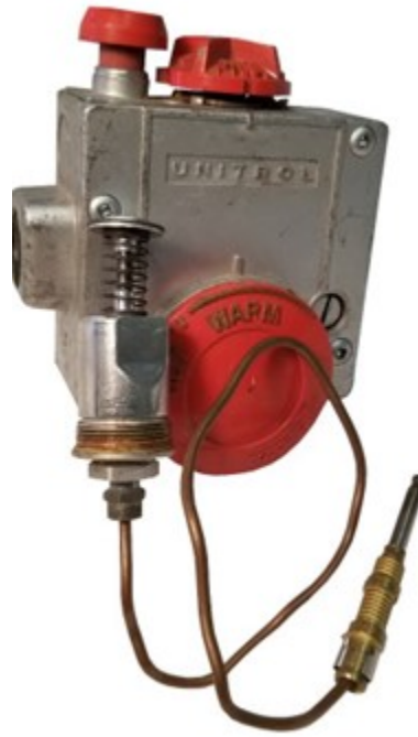
Figure 2 Thermocouple connected to the removed safety shutoff valve
