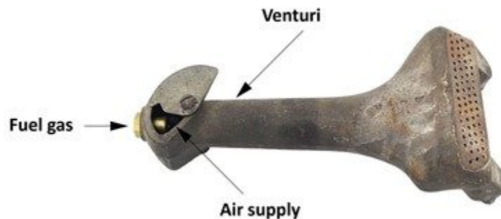
Figure 1 Atmospheric burner
