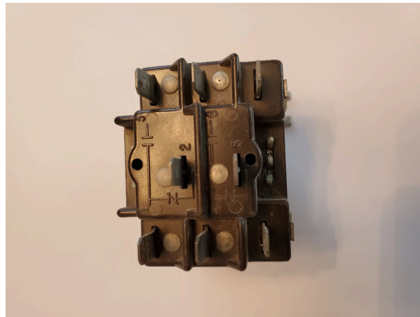
Figure 6 Honeywell DPDT relay with 24VAC coil
