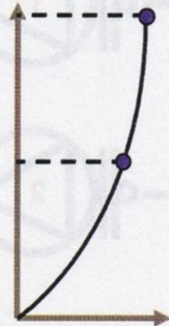
Figure 27 Two pumps in series will double the pressure, with unchanged flow rate
