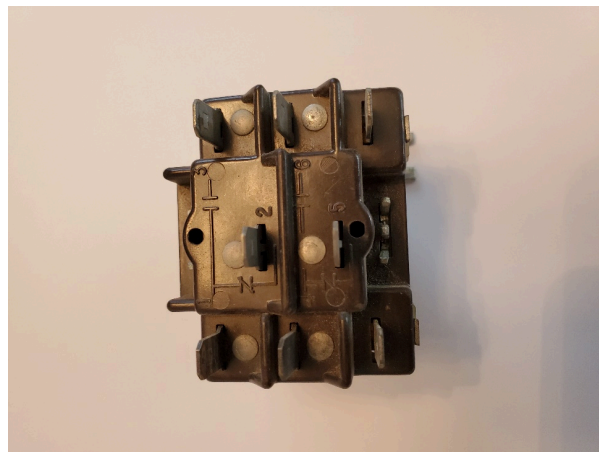
Figure 6 Honeywell DPDT relay with 24VAC coil
