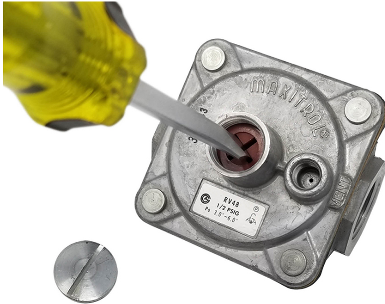
Figure 25. Turning adjusting screw
