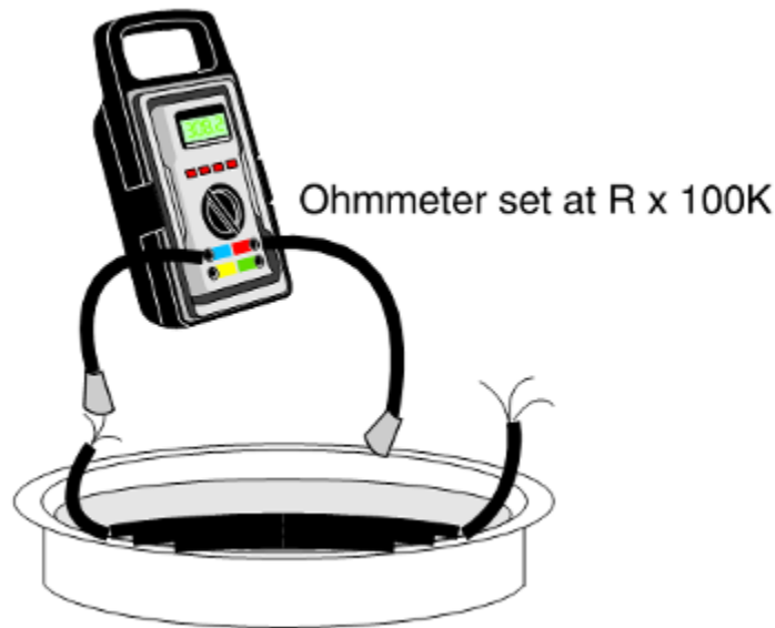
Figure 74. Cable leakage test
