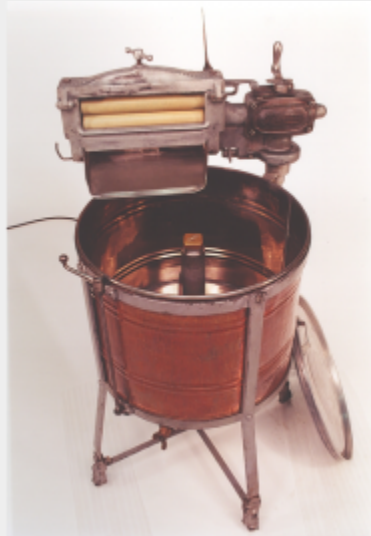
Figure 8.23 A pre-WWII washing machine produced by Beatty Brothers. Note the wringer – or mangle – in which children’s fingers are going to get squished.
